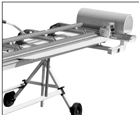
STEP 2 Dispense coil to your desired length along the length of your brake.
