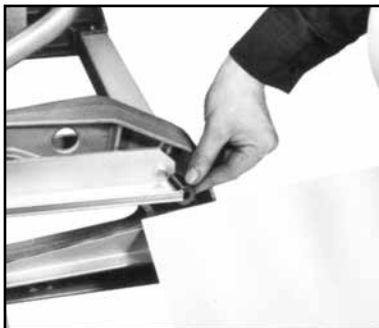
Plastic Coil Guards provided. Install as indicated. Protects Coil from marring.
