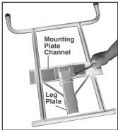
Position leg plates into mounting plate channels, align holes and install nuts and bolts provided.
