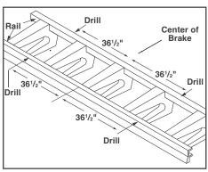
2 Invert Brake. From center of Brake, measure outward along each rail 36<sup>1</sup>/<sub>2</sub>" and drill one pilot hole in center of each rail using an 11/64" drill bit.
