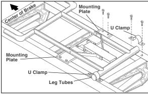
3 Set legs onto Brake with leg tubes near drilled pilot holes. Place "U" clamps over leg tubes, align holes and install sheet metal screws. Drill remaining holes through clamps and install screws. Install screws also in mounting plates as shown.
