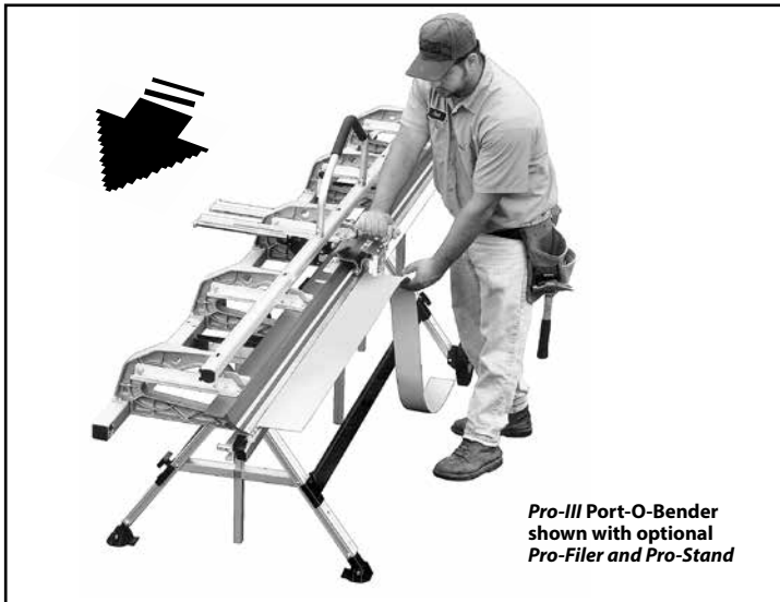
Figure 3. Use proper technique to push CUT-OFF through the material with a smooth, constant motion from right to left. Do not stop in the middle or cut with a back and forth motion. Use a piece or two of scrap material to practice.
